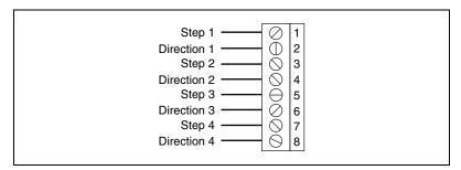
Figure 21. Step and Direction Terminal Block Pin Assignment
